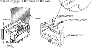
The panel latch should be engaged in the farthest forward slot possible. To achieve a proper seal, tighten the latch screws evenly until the unit is snug in the panel (Torque to approx. 28 to 36 in-oz [0.202 to 0.26 N-m]). Do not overtighten the screws.
