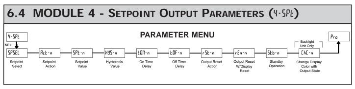
The Setpoint Output Parameters are only active when an optional output module is installed in the meter.
