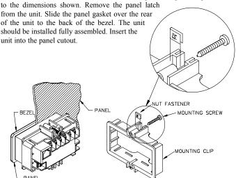
While holding the unit in place, push the panel latch over the rear of the unit so that the tabs of the panel latch engage in the slots on the case. The panel latch should be engaged in the farthest forward slot possible. To achieve a proper seal, tighten the latch screws evenly until the unit is snug in the panel (Torque to approx. 28 to 36 in-oz [0.202 to 0.26 N-m]). Do not over-tighten the screws.
