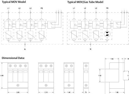
Mounting: Symetrical rail EN50022/DIN 46277-3 I/O Connections: By screw terminal 4-25mm<sup>2</sup> by connection bus
