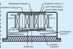
snap it into a closed position against Core B. The armature remains in this position upon removal of power from Coil A, but will snap back into position A upon energizing Coil B. Since operation depends upon cancellation of a magnetic field, it is necessary to apply the correct polarity to the relay coils as indicated on the relay schematic.
