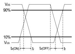
Fig. 18: switching time waveforms
