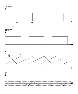
Fig. 4: Current ripple cancellation for output
