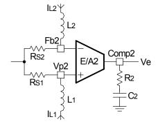
Fig. 22: The Compensation network for current loop
