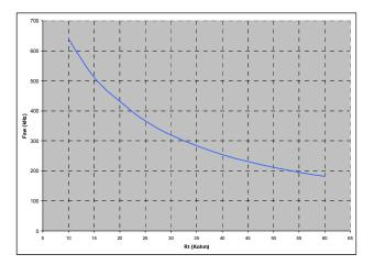
Fig. 16: Switching Frequency vs. External Resistor (Rt)
