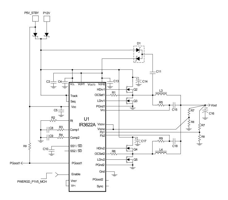
Fig. 25: Application circuit for FBD P1V8 VREG(40A) P5V\_P12V\_STBY
