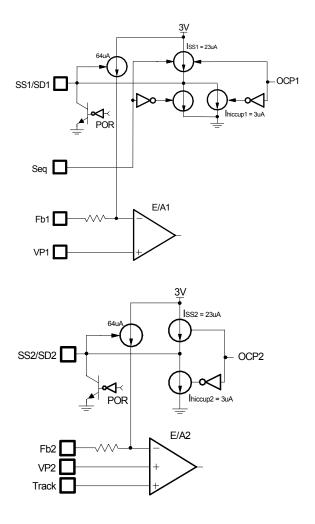
Fig. 7: Soft-Start circuit for IR3622A
