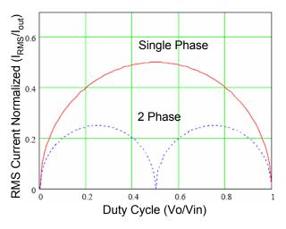
Fig. 5: Input RMS value vs. Duty Cycle
