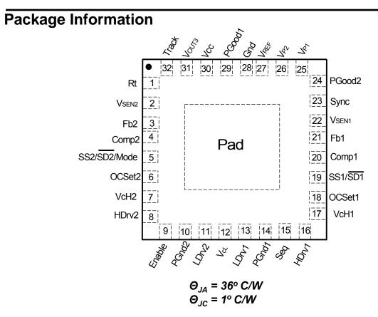
\*Exposed pad on underside is connected to a copper pad through vias for 4-layer PCB board design
