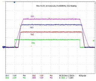
Fig. 10: Ratiometric Power Up / down
