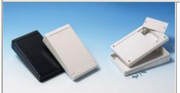
ABS enclosure with a recessed operating area for membrane keyboards. Base and cover have integral PCB guides and mounting studs. Matt surface finish. Fixed by four screws. Recessed operating area 132 x 72 mm. The model with "B" has a battery compartment for two 1.5V mignon-cells or one 9V flat battery.
