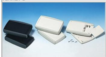
ABS enclosure with new soft-touch contoured shape. By utilising multi-shot moulding technique, Teknet features an ergonomic design of elastomer grips (TPU) on the side of the case. Battery compartment for two 1.5V mignon-cells or one 9V flat battery. Matt surface finish. Closing by four screws.
