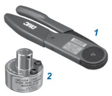
For crimping size #16 shield sleeves. These mil spec approved tools feature a ratchet mechanism to prevent damage from overcrimping. Check calibration with M22520/3 gage.
