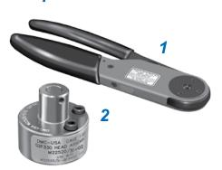
For crimping size #12 shield sleeves. These mil spec approved tools feature a ratchet mechanism to prevent damage from overcrimping. Check calibration with M22520/3 gage.
