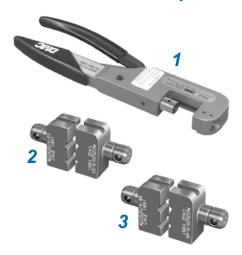
Parallel action tool for use with hex crimp dies. 11 inches OAL, 2.0 pounds. Anodized aluminum frame, steel mechanism, plastic handles. Includes tool for die set removal. Accepts all M22520/5 die sets.
