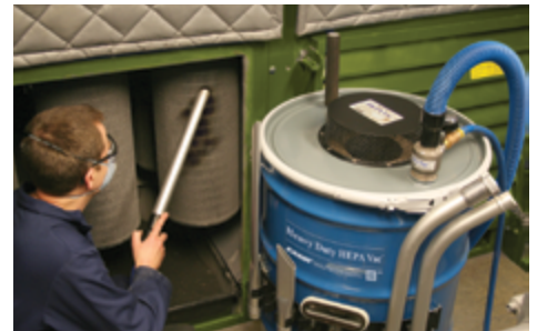
A clogged filtering system for a buffing booth is quickly cleaned and put back into service using the Heavy Duty HEPA Vac.
