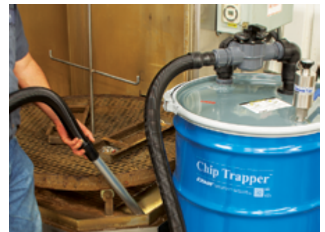
Chip Trapper filters out solids from parts washer fluids.
