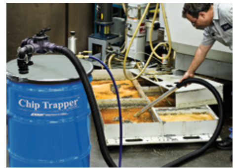
The Chip Trapper vacuums dirty coolant and chips into the drum.
