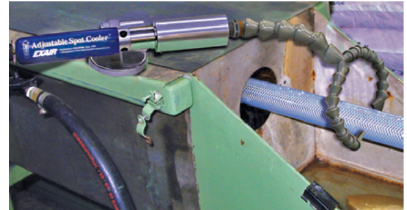
PVC hose is cooled at the exit of an extruder so it can be coiled immediately.
