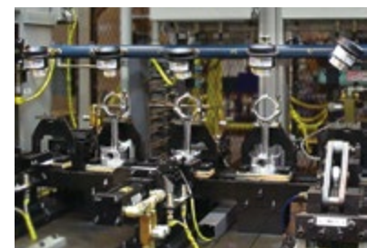
(5) Model 120022 2" (51mm) Super Air Amplifiers cool truck pistons.
