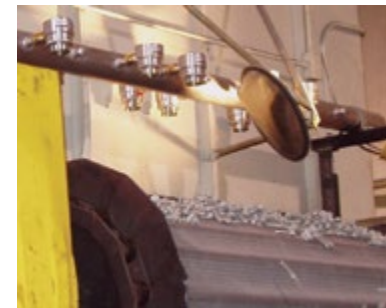
Metal parts are dried using a series of Model 6042 2" (51mm) Adjustable Air Amplifiers.
