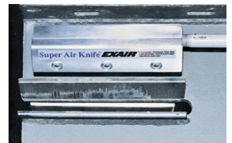
With a 40:1 air amplification ratio, a high volume of airflow is the result from minimal air input to keep linear induction motors from overheating.
