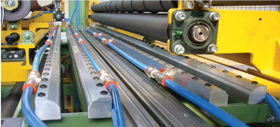
A series of Full-Flow Air Knives “float” layers of plastic film in the confined space of the machine.
