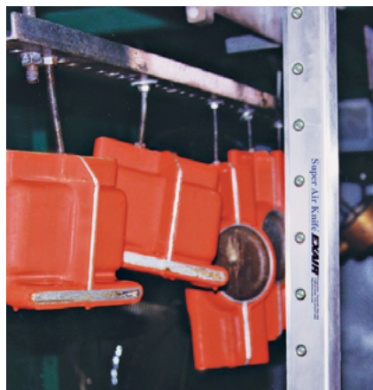
A Model 110018 18" (457mm) Super Air Knife cools molded plastic following dip molding.
