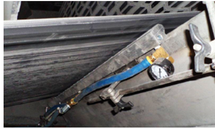
A Model 110048PKI 48" (1219mm) Super Air Knife with Plumbing Kit installed uses EXAIR's Universal Air Knife Mounting System to maintain proper position for removing dust on a conveyor belt and eliminate carryover accumulation.
