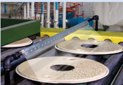
Model 110054 54" (1372mm) Super Air Knife dries stamped parts that exit a washer.
