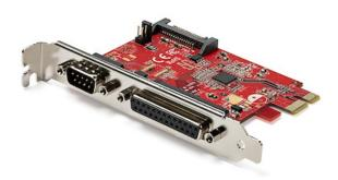
This PCIe Parallel and Serial Combo Card installs into a single PCI-Express x1 slot in your computer, and adds a DB25 IEEE 1284 parallel port and DB9 RS 232 serial port to your system. The PEX1S1P950 is the latest version of our popular PEX1S1P952 combo card.
