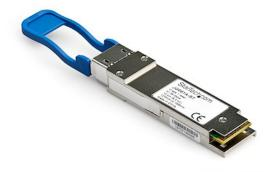
The JG661A-ST is a HPE JG709A compatible fiber transceiver module that has been designed, programmed and tested to work with HPE brand switches and routers. It delivers dependable 40 GbE connectivity over fiber cable, for 40GBASE-SR4 compliant networks, with a maximum distance of up to 300 m (984 ft).
