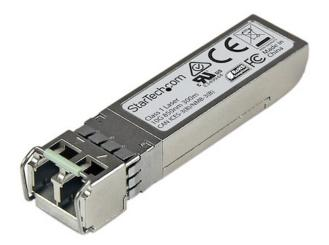
The SFPP10GESRST is a Palo Alto Networks XBR-000182 compatible fiber transceiver module that has been designed, programmed and tested to work with Palo Alto Networks brand switches and routers. It delivers dependable 10 GbE connectivity over fiber cable, for 10GBASE-SR compliant networks, with a maximum distance of up to 300 m (984 ft).
