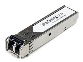
The 0231A0A8-ST is a HPE 0231A0A8 compatible fiber transceiver module that has been designed, programmed and tested to work with HPE brand switches and routers. It delivers dependable 10 GbE connectivity over fiber cable, for 10GBASE-LR compliant networks, with a maximum distance of up to 10 km (6.2 mi).
