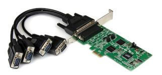
The PEX4S232485 4 Port PCI Express PCIe Serial Combo Card - 2 x RS232 2 x RS422 / RS485 lets you add two RS232, and two RS422/485 serial ports to your PC through a PCI-Express expansion slot.
