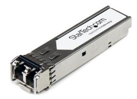
The EW3P0000558-ST is a Citrix EW3P0000558 compatible fiber transceiver module that has been designed, programmed and tested to work with Citrix brand switches and routers. It delivers dependable 10 GbE connectivity over fiber cable, for 10GBASE-LR compliant networks, with a maximum distance of up to 10 km (6.2 mi).
