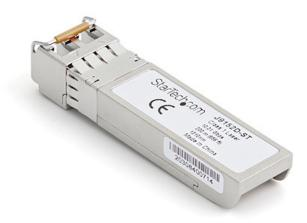
The J9152D-ST is a HPE J9152D compatible fiber transceiver module that has been designed, programmed and tested to work with HPE brand switches and routers. It delivers dependable 10 GbE connectivity over fiber cable, for 10GBASE-LRM compliant networks, with a maximum distance of up to 200 m (656 ft).
