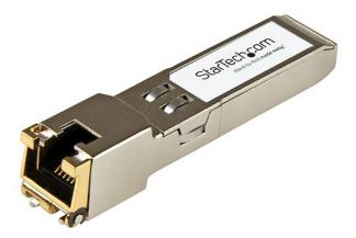
The AR-SFP-1G-T-ST is an Arista Networks compatible copper transceiver module that has been designed, programmed and tested to work with Arista Networks brand switches and routers. It delivers dependable 1 GbE connectivity over copper cable, for 10/100/1000BASE-TX compliant networks, with a maximum distance of up to 100 m (328 ft).
