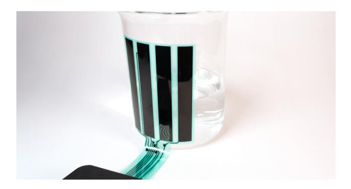
The Trent Evaluation Kit allows you to explore LAIIER's Trent technology and test the Trent Sensor against your use cases. It contains the Trent Evaluation Board and LAIIER's capacitive Trent Sensors.
