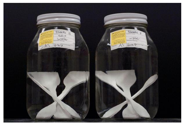
Figure 2: 3M performs long-term fresh water and salt water laboratory immersion testing on marine sealants
