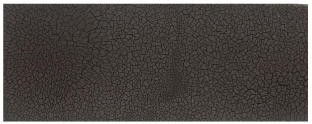
Figure 1: Cracks in the sealant can often be an indication of premature degradation.
