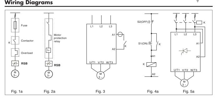
The motor controller provides by-passing of the semiconductors during running operation. Therefore the semiconductors can only be damaged by short-circuit currents during ramp-up and ramp-down. Please note that the motor controller does not insulate the motor from the mains.
