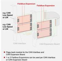
Expands the existing CAN High Speed channel by a switchable CAN Low Speed channel or a LIN channel
