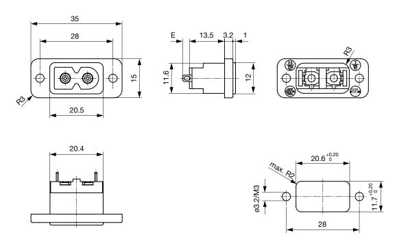
E: Solder terminals long: 7.3 mm (L=8.5 mm)
