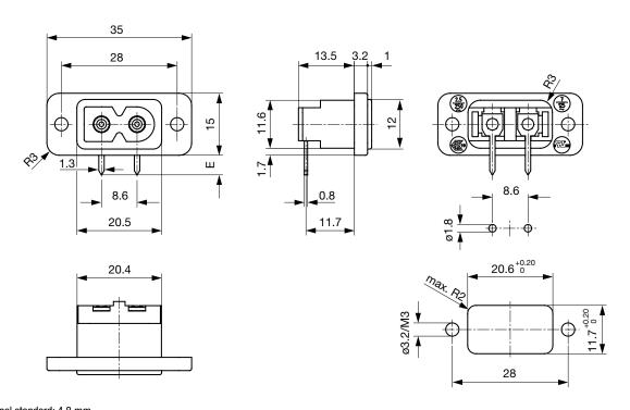
E: PCB terminal standard: 4.8 mm E: PCB terminal short: 3.2 mm E: PCB terminal long: 5.9 mm
