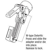
**Important:** W-type dies must be locked into place or the die detents will be damaged.
