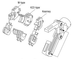
**Important:** W-type dies must be locked into place or the die detents will be damaged.
