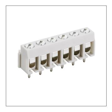
Screw terminal block, clamp with wire protector, upright version, consecutive placement without loss of pitch contact pitch 5.0 mm
