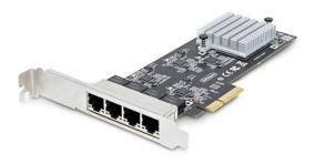
This quad-port 2.5 GbE network interface card (NIC) features an Intel I225-V chipset with Intel vPro technology, to enhance performance and data integrity across four 2.5G ethernet connections. The variable multispeed options (2.5/1Gbps and 100/10Mbps) enable support for both new and legacy network hardware. Utilize existing Cat5e or CAT6 cabling infrastructure while adding NBASE-T (802.3bz) compatibility for seamless integration.
