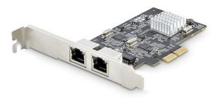
This dual-port 2.5 GbE network interface card (NIC) features an Intel I225-V chipset with Intel vPro technology, to enhance performance and data integrity across two 2.5G ethernet connections. The variable multispeed options (2.5/1Gbps and 100/10Mbps) enable support for both new and legacy network hardware. Utilize existing Cat5e or CAT6 cabling infrastructure while adding NBASE-T (802.3bz) compatibility for seamless integration.
