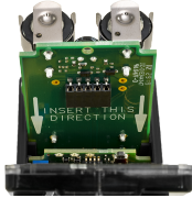
Figure 4: Q45 battery board
