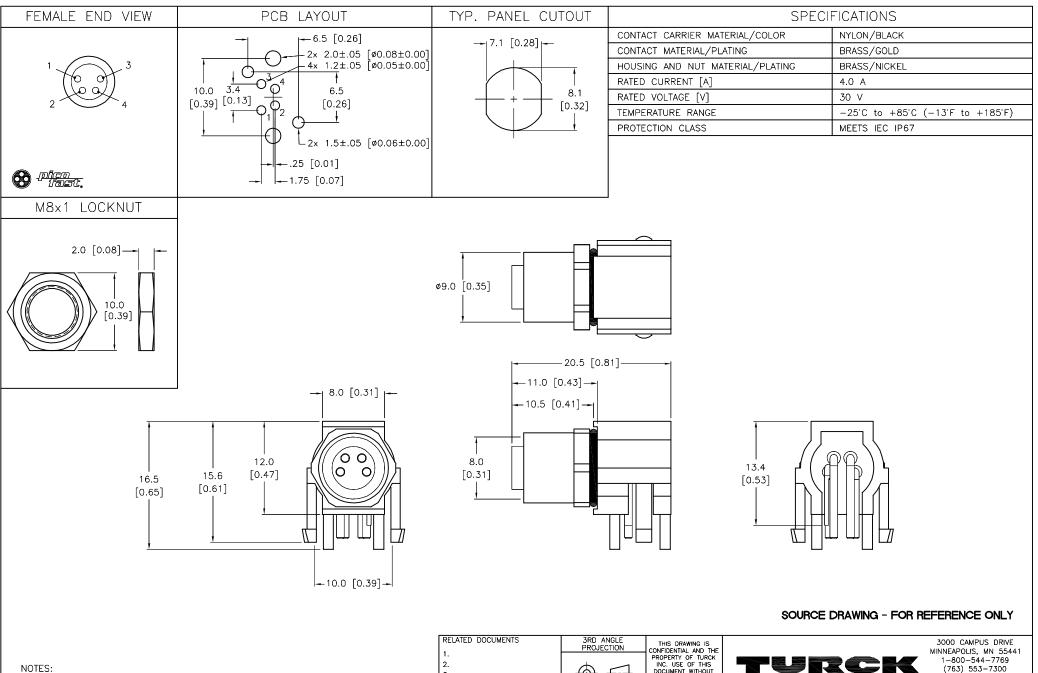
1. RECOMMENDED THICKNESS OF PCB 1.5mm.
