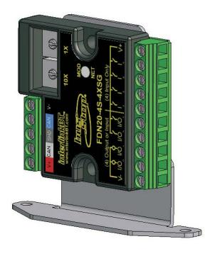
The *busstop*® station provides a connection for 8 I/O points. The first 4 points can be either inputs or outputs. The other 4 points are inputs only. All inputs and outputs are powered by DeviceNet $^{\text{TM}}$ . This is ideal for small systems that don't require auxiliary power.
