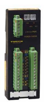
This station provides a connection for 16 I/O points. All pointa can be either inputs or outputs. All inputs and outputa are isolated from DeviceNet. To use an I/O point as an input, simply leave the corresponding output bit off. To use an I/O point as an output, simply turn on the corresponding output bit. The output will switch on high. Note that this will in turn cause the corresponding input bit to turn ON. If the corresponding input does not turn on, the output is shorted.
