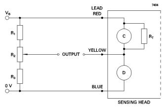
$R_1$  =  $R_3$  = 500 to 5000  $\Omega,~R_2\cong R_1/5$   $R_2$  provides zero adjustment and may be omitted if not required.
