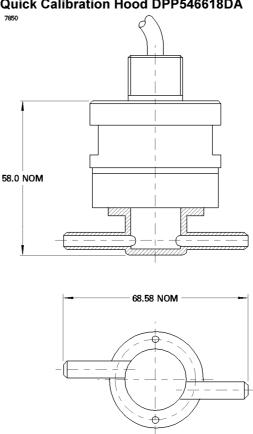
Quick Calibration Hood is constructed from polypropylene, and provides a convenient means of supplying test gases to the VQ600 in the field, for calibration and checking purposes. The assembly push-fits into the central gas access recess of the head, and is designed to accommodate 6 mm ID or 1/4" flexible tubing.
