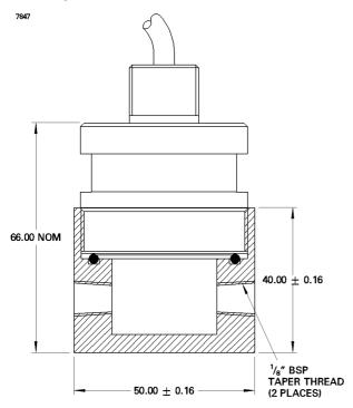
The Flow Cap allows the VQ600 to be used in applications where it is to be aspirated permanently with a pumped or pressurised sample. The cap is made of 316 stainless steel and can be used in a variety of applications involving pumped sampling analysis or detection systems.
