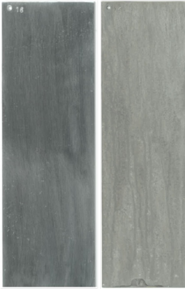
Sample 16: Polished and etched Aluminium 6061-T6, before testing (left) and after testing (right).
