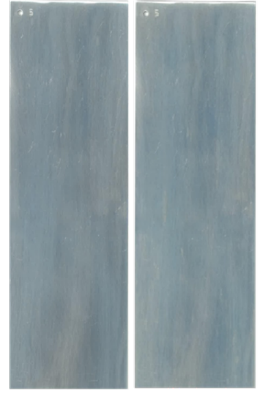
Aluminium 6061-T6 sample treated with Surtec 650 passivation, prior to testing (left) and after testing (right).
