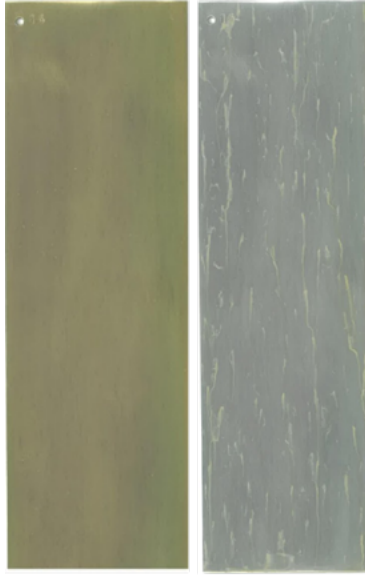
Sample 14: Aluminium 6061-T6 Passivated with Alocrom 1200. Before (left) and after (right) salt fog testing.
