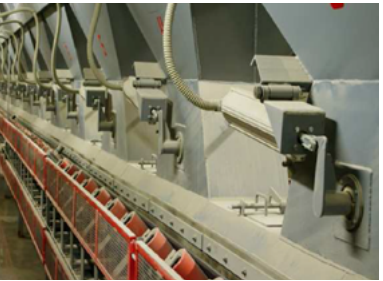
Control of silo discharge in fertilizer processing
