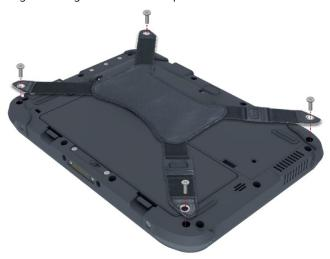
4. Insert four M3x8 flat head screws and tighten them.
