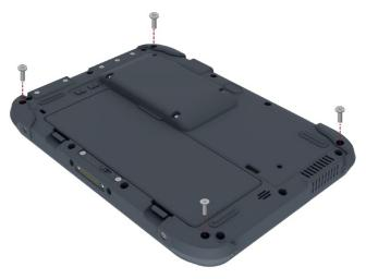
3. Align four rings on the hand straps to screw holes on the tablet.
