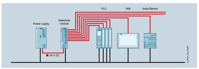
As an electronic monitor, the SITOP selectivity module switches faulty 24 V DC load circuits off immediately, and continues to supply the other loads without any interruption.
